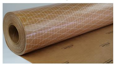
ZERUST® ICT®430-35PCR Poly Coated Reinforced VCI Paper is a high-quality 35# kraft paper that is saturated on one side with proven ZERUST® corrosion inhibitors and laminated with a 3/4 mil polyethylene layer and fiberglass scrim on the backside to provide superior strength. Place the plain kraft paper side facing the metal surface to allow the powerful vapor corrosion inhibitors (VCI) to protect ferrous and non-ferrous metal coils.
