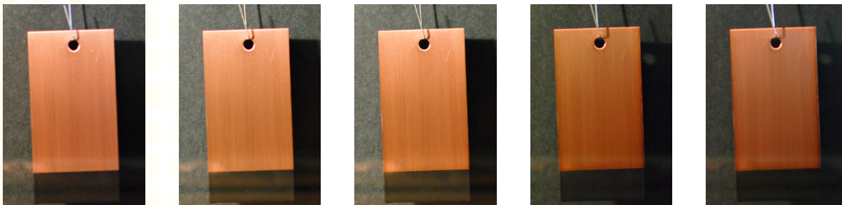
Panel protected by ActivPak® in H 2 S sulfur gas environment. (2-18 ppm)
