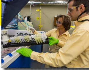
**Description:** Testing of a specimen (components coated with fluids, or packaged in material) in a humidity chamber in accordance to ASTM D1735 for 30 days. Results will be sent via email and mail to client at the end of testing. Up to eight (8) fluids or packaging materials per test.
