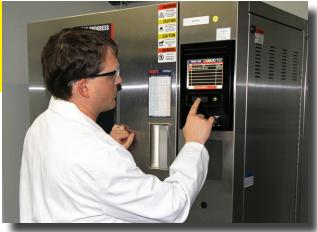
**Description:** Testing of a specimen (components coated with fluids, or packaged in material) in a cyclic temperature and humidity chamber in accordance to IEC 60068-2-30 for 15 days. Results will be sent via email and mail to client at the end of testing.
