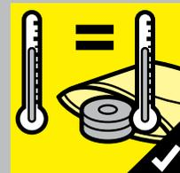
When packing, the temperature of the parts should be near room temperature to avoid condensed moisture.
